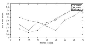
Fig. 7 End to end delay vs number of nodes in column mobility
