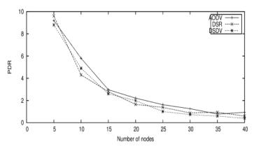
Fig. 6 Packet delivery ratio vs number of nodes in random way point mobility model
