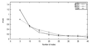
Fig. 5 Packet delivery ratio vs number of nodes in group mobility model
