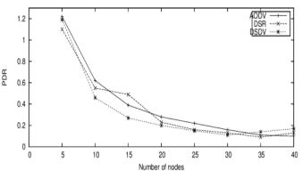
Fig .4 Packet delivery ratio vs number of nodes in column mobility model
