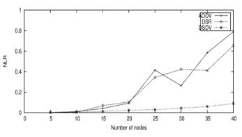
Fig. 10 Normalized routing load vs number of nodes in column mobility
