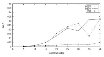
Fig. 11 Normalized routing load vs number of nodes in group mobility
