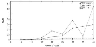
Fig. 12 Normalized routing load vs number of nodes in random way point mobility
